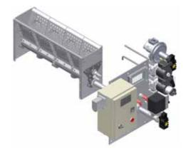
The burner consists of a plate to which the mixing head is fixed (positioned in the centre of the duct). Outside the plate there are the control board with flame control equipment, the interception and regulation gas train and the flame detector.
