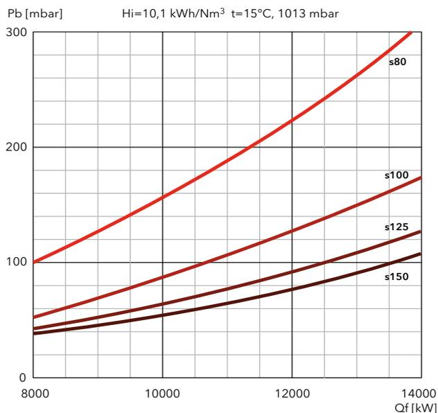
**PERDITE DI CARICO [TESTA BRUCIATORE + RAMPA GAS] (mbar)**
